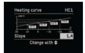
Vitotronic 200 HO1A heating curve
