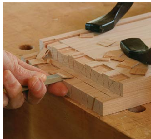
First chip is the slimmest. Remove a thin chip of waste with a tap on a horizontal chisel, and you'll have a \frac{1}{16} -in.-deep square shoulder. To chop out the rest of the waste, hold the chisel just off vertical—tilted toward you—and use harder mallet blows. This undercuts the joint, leaving the shoulder intact.
