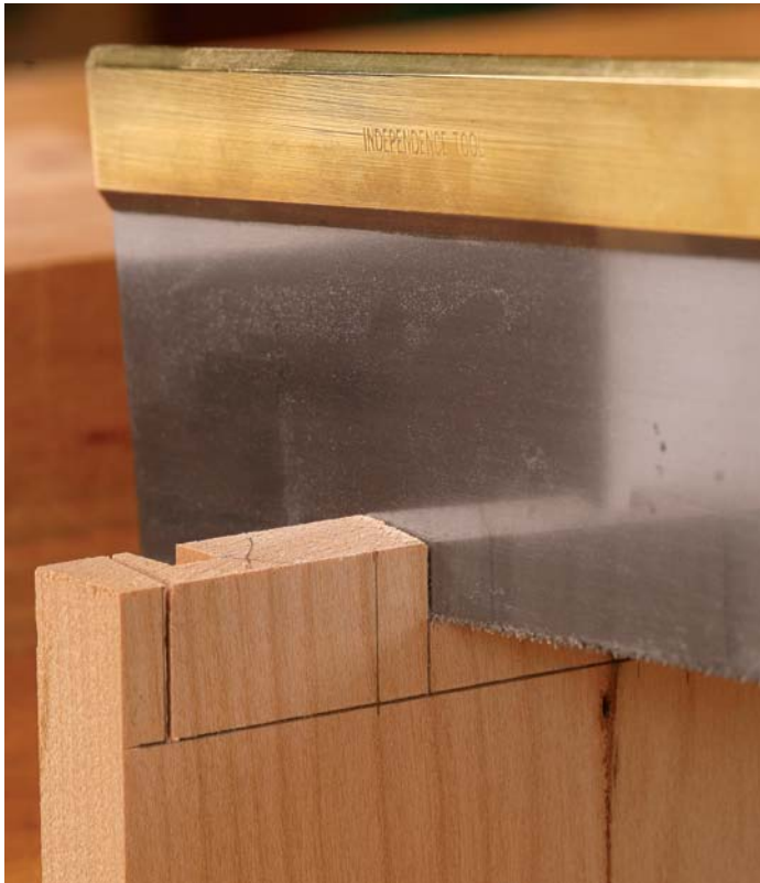
Down to the line. Your kerf should be right on the knife and pencil lines. Mark the waste with Xs to avoid mistakes.
