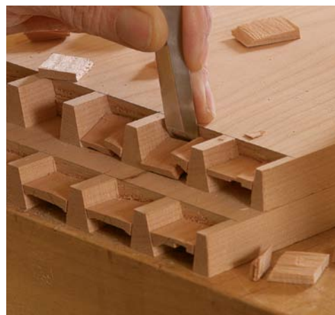
Same sequence on side two. After chopping to the middle of the pin boards, flip them and use the same techniques to establish a square shoulder and chop away the waste on the other side. Lighten up at the end to avoid damaging the shoulder below.
