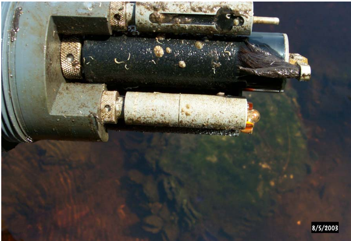
YSI 6600 Extended Deployment Data Sonde Probes
