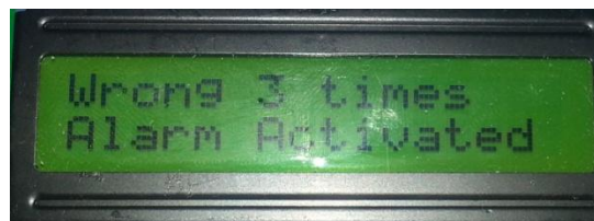
Figure 41: Output of entering 3 times of wrong password
