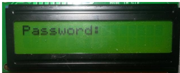
Figure 36: Keypad output (password) at LCD display
