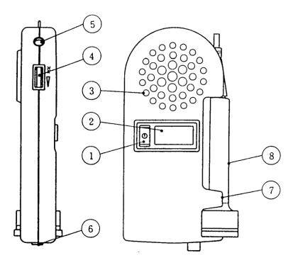
① Power switch : The switch is used to turn power ON or OFF.
