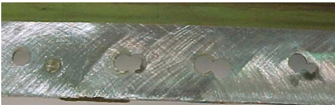
Figure 14. Improper Drilling Workmanship and Failure to Follow Correct Repair Procedure
