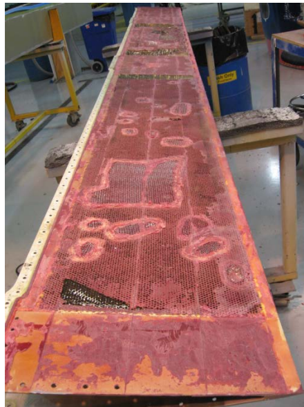
Figure 8. Uneven Film Adhesive Thicknesses May Have Been Caused by Tooling Contour Inaccuracies
