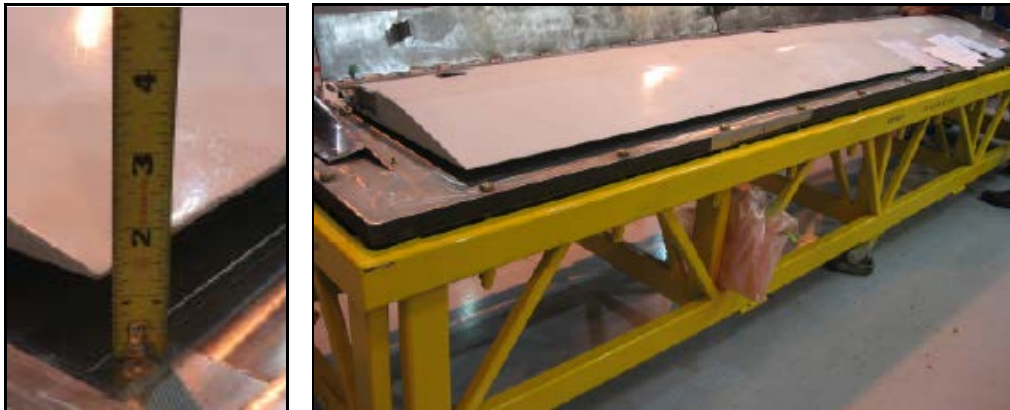
Figure 1. Overhauled Flap Assembly Placed on Tooling That Served as a Check Fixture
