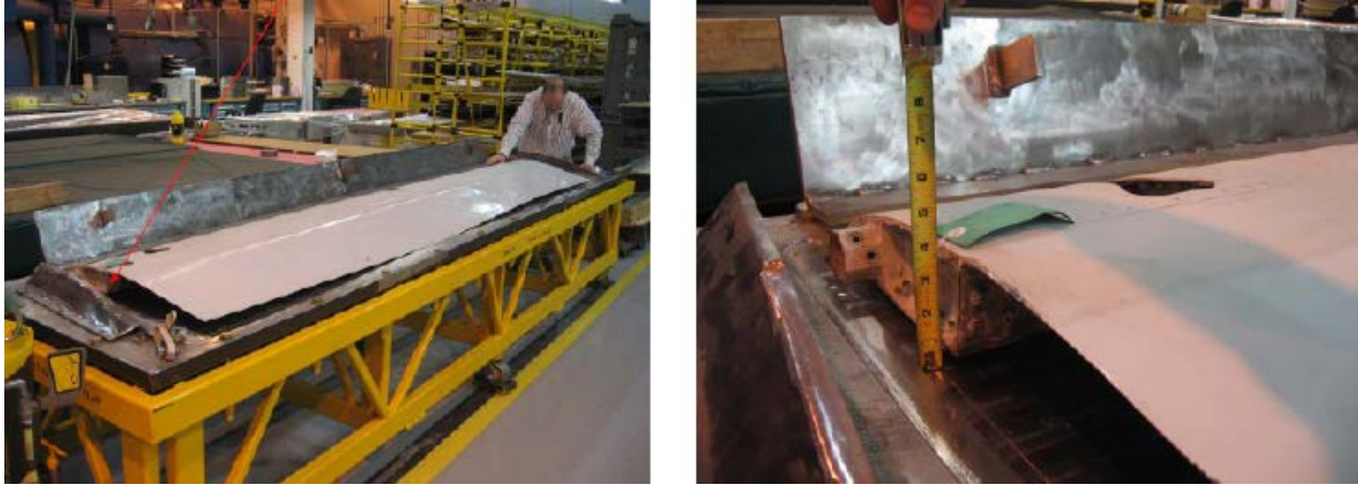
Figure 4. Out-of-Contour Condition of the Spar Resulting From the Use of Improper Tooling
