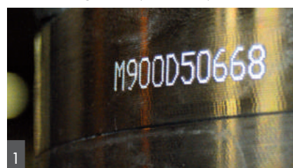
(1) Marking of a cylindrical part in bronze
