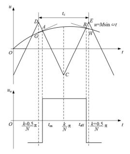
Figure 4. Double tangent sampling method.
