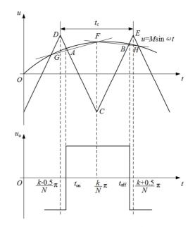
Figure 3. Secant sampling method.
