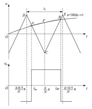
Figure 2. Tangent sampling method.
