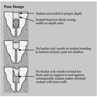
Figure 3 – Joint Design Considerations: *Dow Corning* 890-SL Silicone Joint Sealant
