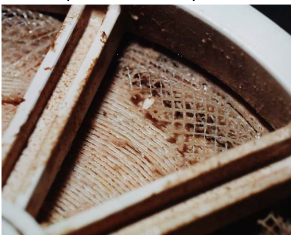
Figure 8.11 High pressure drop due to biofouling has pushed out the feed spacer
