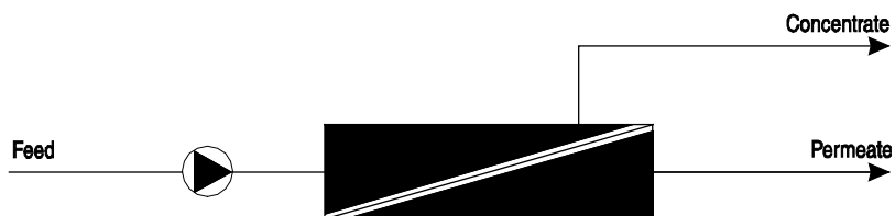
Figure 3.1 Continuous RO process
