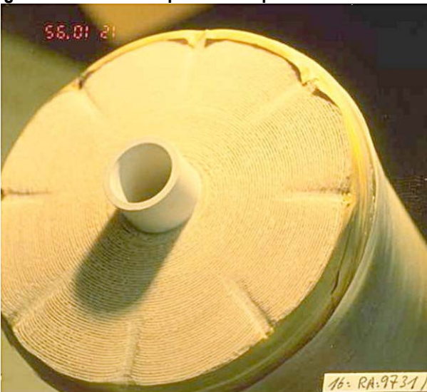
Figure 8.9 The endcap has been pushed off
