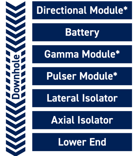
Figure 12: Downhole Trial MWD Tool String Configuration
