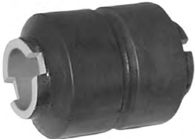
Bushing; 1 1/2" I.D. x 3 1/8" O.D. x 4 7/16" Lg; Included in 334-243 Equalizer Bolt and Bushing Assy.; w/ Slots; Models: Various
