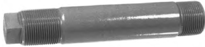
Shaft, Standard Equalizer; 1 1/2" O.D. x 8" Lg., 1 7/16"-12 Thread BE; Model 101, 101A, 102, 102W
