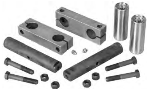
Shackle Kit; 3 9/16" c/c; Incl. (2) 330-186, (2) 327-483, (2) RNK-BM & Hdwe. Front w/4" Springs
