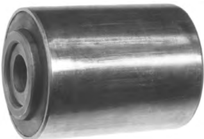
Bushing; 1" I.D. x 3" O.D. x 5 1/4" Lg.; Models Quadraflex, Four Spring Tandem
