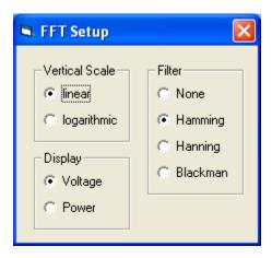
Checking the %FT+option will change the display to frequency domain: The oscilloscope performs a real-time FFT (Fast Fourier Transform) on each captured record. This is a highly useful mode to analyze periodic signals or to find small periodic components (e.g. periodic noise from the power line) hidden in the main signal . it is much easier to see an isolated 60 Hz component (spectral line) in a frequency plot than it is to see it among all the random noise riding on the signal.
