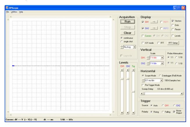
The left side of the display is taken up by the waveform display. On the right side you can see that the controls are grouped in several functional blocks (we will explain each of them in more detail later):
