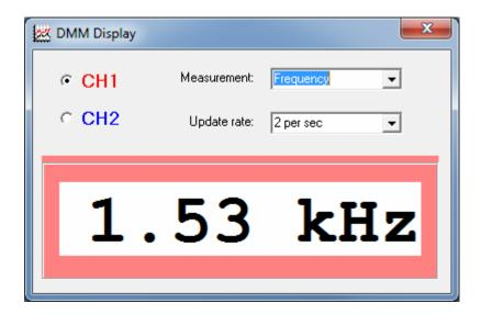
While the automated measurement panel is convenient, sometimes you may want to observe only a specific value. This could be e.g. to trim the frequency or the amplitude of an oscillator. Chances are you do this at some distance from the screen so it is important that the display is large enough to be observable without being right in front of the computer.
