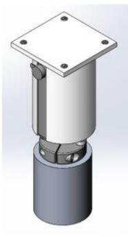
This mechanism will be attached to the fluid handling system and together with the manipulator will unscrew and screw back again the conical tubes' caps.
