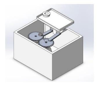
Shaker enclosure protects gear and motor systems
