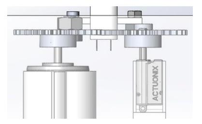
Linear actuator used as gear shifter disengages second gear, causing single orbital motion from single gear and motor
