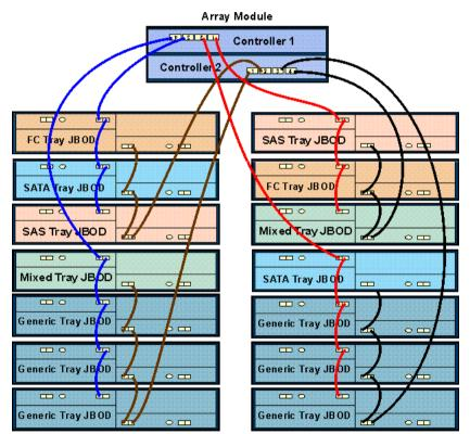
Array Module with Different Drive Tray Types
