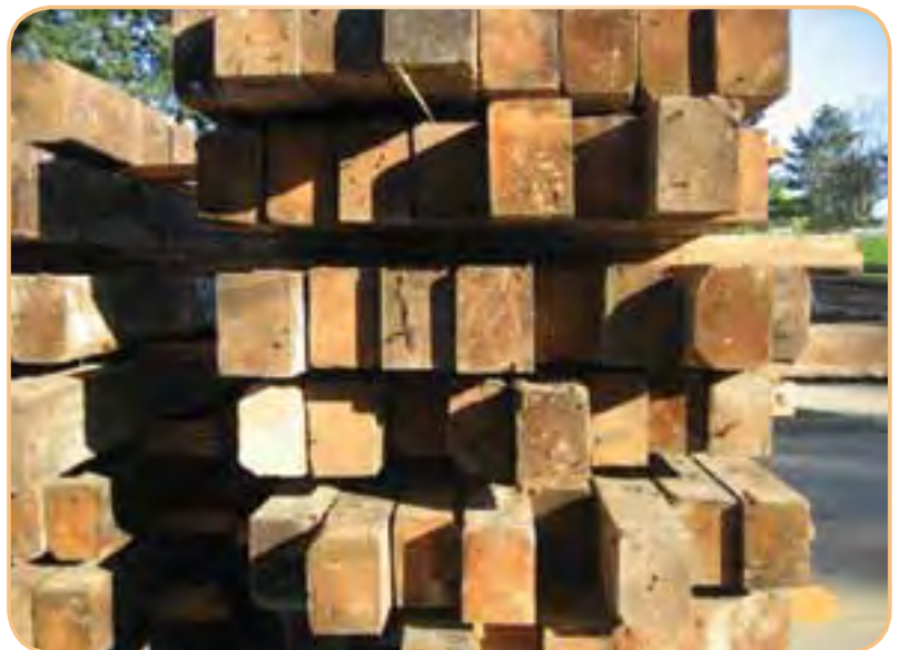
Wood beams from a deconstruction site are salvaged for use in new building construction.
