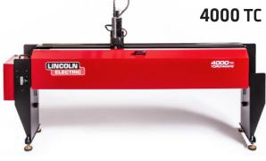
The two-axis tube cutter is capable of cutting and profiling schedule 40 pipe with an outside diameter of 1.5 to 6 inches and a machine cutting envelope of 84 inches. It easily connects to the  $4 \times 00$  series tables with cable connections. The two inch through chuck allows for loading longer pieces of small diameter tubing to reduce scrap. A 45 degree bevel axis is included for automated weld coupon creation.
