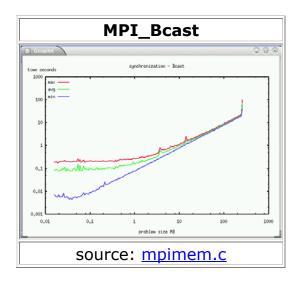
One aspect of the scaling of MPI collectives which is not depicted above is the variability in timings. Highly synchronizing calls of any sort not only show greater average delays at higher concurrency, but also show greater relative variability in the length of delays.
