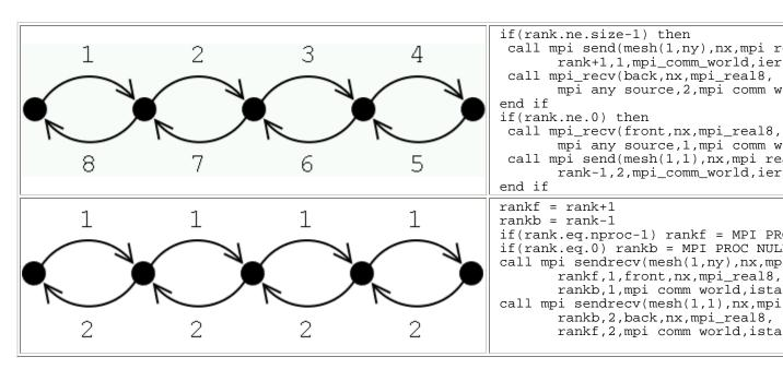
Choose messaging strategies that wait as long as required (but not longer) to initiate the communucation needed for the computation. The above example includes more delays (though blocking MPI) than are required for each node to exchange boundary data with it's neighbors.
