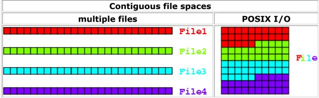
In this case each task does its nbytes of I/O to a separate file or a unique region of a common file.
