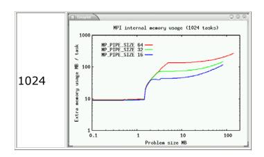
Since there are potential performance penalties when using smaller MPI buffers it is recommended that the use of MP\_PIPE\_SIZE=32 or 16 should be viewed as a workaround for codes running out of memory rather than a standard programming practice for large concurrency jobs.
