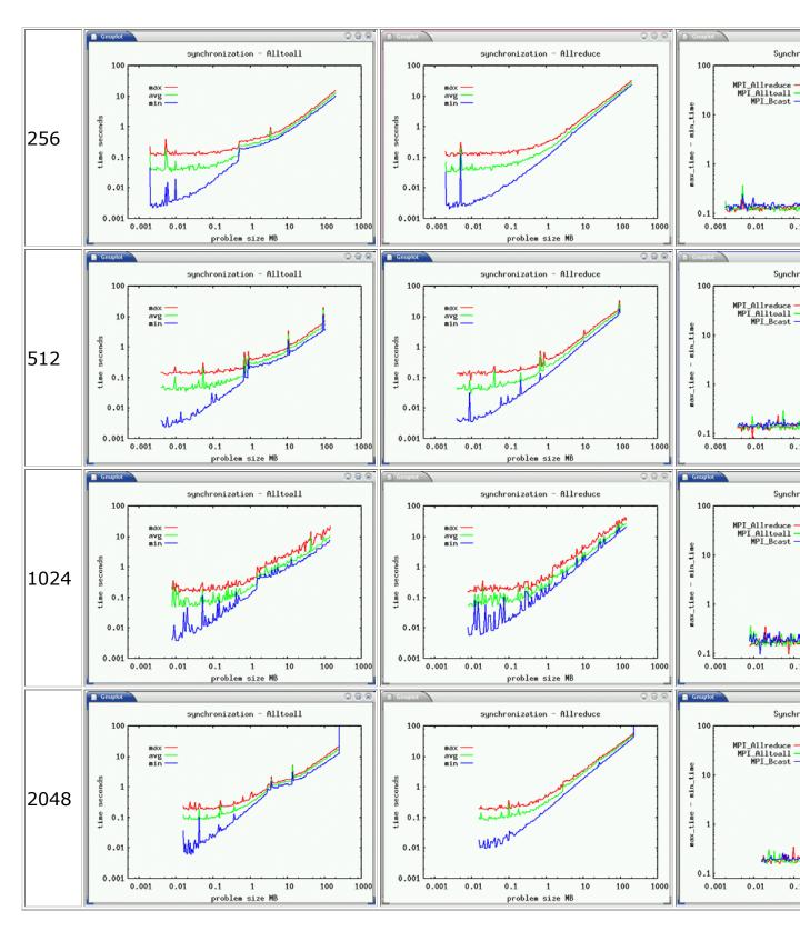
MPI\_Bcast which is not fully synchronizing does not show as large or as varied timings. Though a broadcast and a all-reduce are quite
