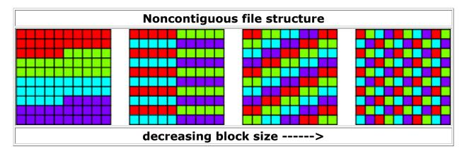
For suffciently small block size the metadata and file locking tasks required from GPFS are expected to impede performance. Each of the I/O operations, taken individually is more complicated for the filesystem than if coordianted at a global level by MPI-I/O. For this reason MPI-I/O should be able to provide the benefit when the block size is small enough.
