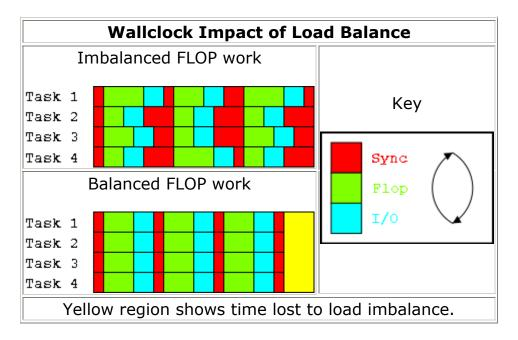
In practice the MPI portion of the code could be in in either or both of the I/O or Sync parts of the code. While load imbalance can occur in these parts of a code (particularly if the I/O involves disk activity), the most important path to enforcing load balance is in evenly partitioning the problem space across the PEs.
