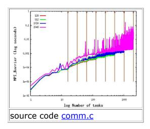
The impact of concurrency on synchronization times is dramatic, spanning four orders of magnitude. The IBM SP is a cluster of independently scheduled instances of AIX, for this reason it grows increasingly unlikely that at a given moment all the nodes involved will be ready to complete a synchronizing operation.
