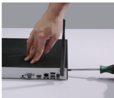
⑥ Put the cover back, and secure the screws of the cover
