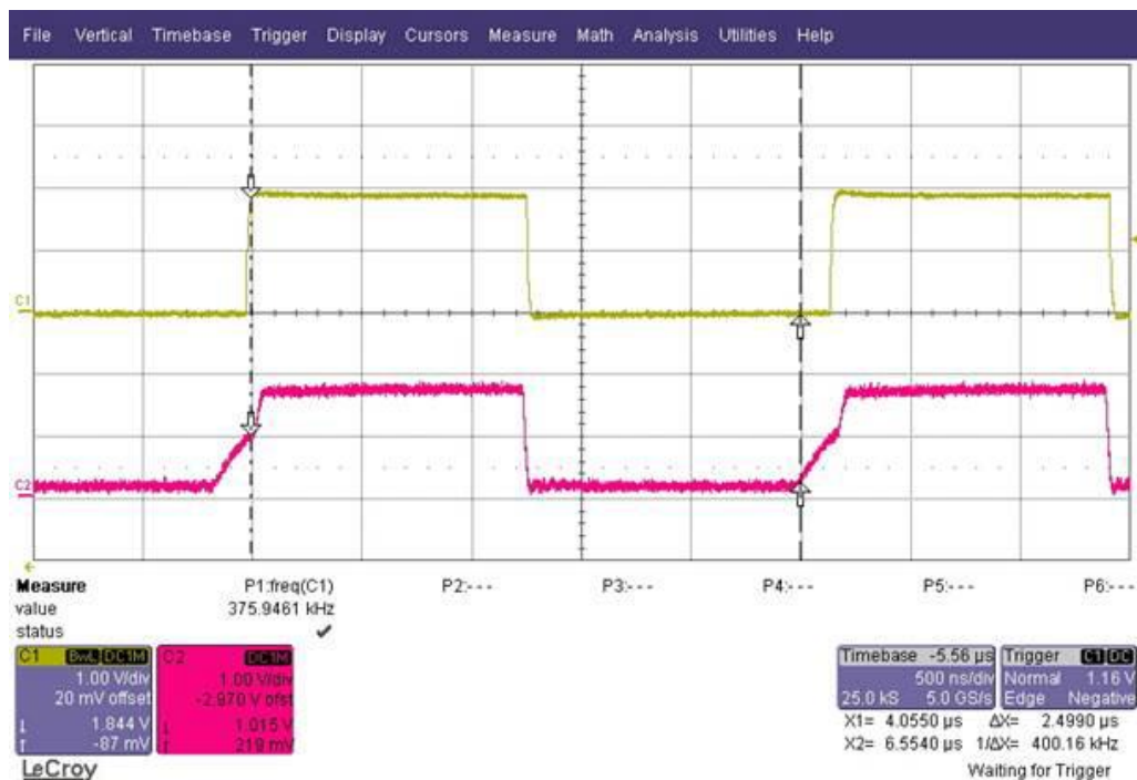
Figure 4-2 Output clock is 400 kHz due to excluded rise time
