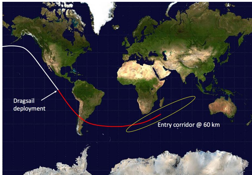
Fig. 8. Dragsail deployment can be used to initiate spacecraft reentry, thereby constraining the entry corridor to a targeted region.
