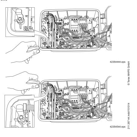
Connecting the flat cable from the radio receiver to the controller card of the rope hoist control system
