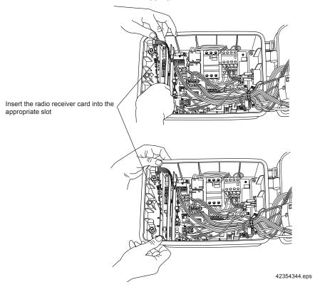
Fix the radio receiver card in the electric equipment cover by means of the two screws
