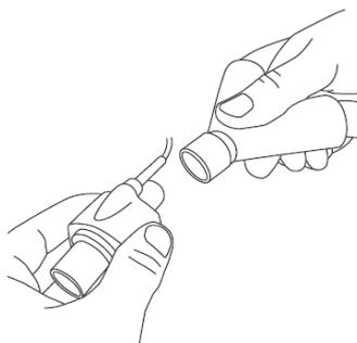
5. Connect the 15mm female connector of IRMA/airway adapter to the patient's endotracheal tube.
