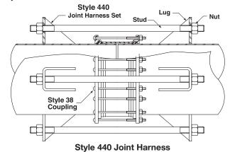
Used in conjunction with a Dresser Style 38 coupling on steel pipe installations
