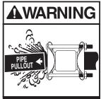
When pipe pullout could occur, pipe joint MUST be anchored. Failure to anchor pipe joint could result in escaping line content and cause property damage, serious injury or death.
