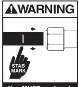
You MUST mark and stab the pipe into the fitting to the proper stab depth. Failure to do so could result in escaping line content that could cause property damage, serious injury or death.
