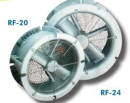
Rugged, cast aluminum housing and fan blade make these fans ideal for hazardous locations and demanding ventilation projects. The RF design utilizes action-reaction principles; compressed air is discharged through nozzles located at the tip of the fan blade providing extremely efficient, high-volume, low-maintenance air movers.
