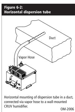
Locate the CRUV humidifier near an electric power source, a water supply, and a drain. Verify that sufficient room is provided for a water seal in the drain piping. See Figures 8-1 and 9-1).
