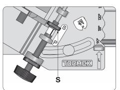
After grinding the primary facets, the drill holder is moved forward to a second stop  $\mathbf{S}$  for grinding the secondary facets, which gives the drill a 4-facet point.
