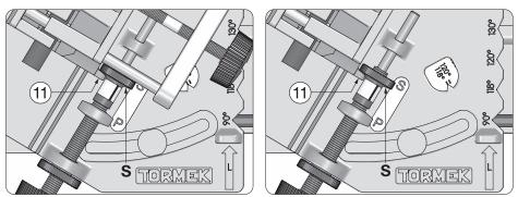
Grind the two secondary bevels alternately until the lug (11) touches the stop nut **S** on both sides. Make the final grindings carefully and check that the facets are symmetrical and form a point.
