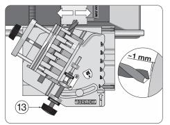
Adjust the setting screw (13) so that the drill is approx. 1 mm (0.04") from the grindstone. Start the machine.
