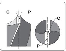
You can tell by the decreasing sound when the primary facets **P** are ground equally. How far they are ground over the centre does not matter. It is important that they are ground symmetrically. The primary facets should meet and form a flat chisel edge, C.
