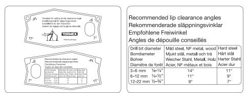
**Clearance angle**. With the Tormek Setting Template you can set the clearance angle to 7°, 9°, 11° or 14°. The Template recommends a suitable angle based upon the drill size and the material to be drilled.
