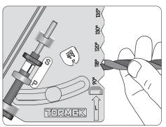
**The point angle.** Measure the existing point angle in the grooves on the Guide or select the angle which is most suitable for the job.
