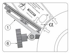
*The clearance angle, a.* Here 7°. Tilt the Base (1) so that both corners of the Setting Template touch the grindstone. Lock it securely with the wheel (6).
