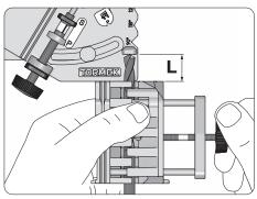
Mount the drill with the protrusion **L** indicated by the stop on the Guide. Lock the drill temporarily.
