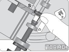
Feed the nut **S** a bit further. Try with  $\frac{1}{4}$  of a turn. One turn is equal to 0.5 mm (0.02").
