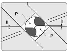
Mount a heavily worn drill turned anticlockwise.
