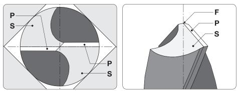
This is how a ground drill should look like. The secondary facets **S** meet the primary facets **P** in the centre. The flat chisel edge has been shaped to a point, **F**.
