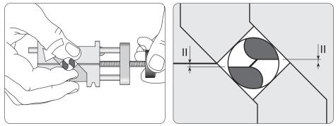
Loosen the wheel and rotate the drill so that the cutting edges are aligned parallel to the horizontal lines on the Drill Holder. Tighten the wheel. The protrusion L does not need to remain exact.
