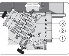
The drill is mounted in a Drill Holder (3) on a Guide (2), which in turn runs on a Base (1). You move the drill across the grindstone – the grinding automatically takes place on the highest spot of the stone.
