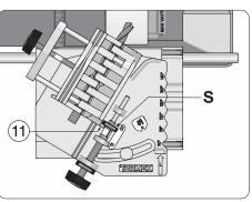
Lift and move the drill holder forwards so that the lug (11) rests on the stop nut **S**.
