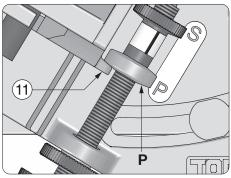
Lift and move the drill holder so the lug (11) touches the stop  ${f P}$ .
