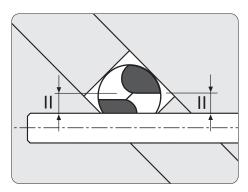
The cutting edges should be parallel to the pin in the Magnifier.
