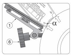
**The clearance angle**. Place the Setting Template according to the image and tilt the base (1) so that the corners of the Setting Template touch the grindstone. Lock it securely with the wheel (6).
