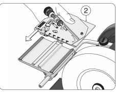
Slide the Guiding Plate (2) into the base plate.
