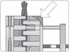
Turn the drill holder so the bevelled side points towards the machine.
