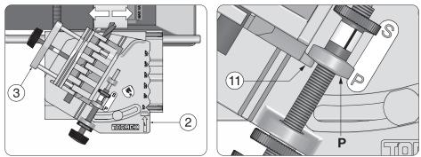
Place the Drill Holder (3) on the guide (2) so that the lug (11) touches the stop **P**.
