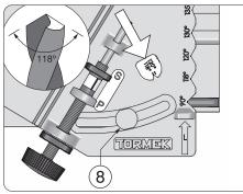
**The point angle**. Set the point angle at 118°. Lock securely with the wheel (8).
