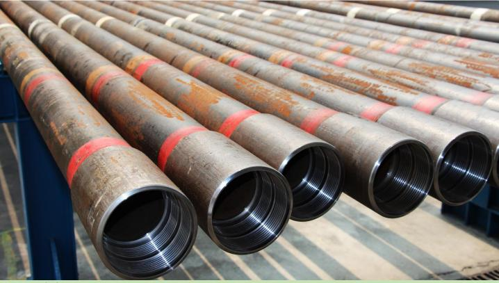
Drill Pipe TS6 Connection Repair
