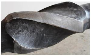
Laser cladding and coating yield high precision and homogeneity in depositing powder onto the base material. The coatings and overlays impart greatly improved performance of the desired characteristics such as: wear resistance, impact resistance, sliding wear, corrosion protection, friction modification and specific electrical properties.
