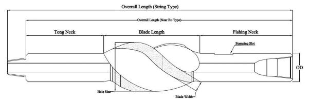
Integral ribs: Milled from the steel body and have no welded or loose parts.
