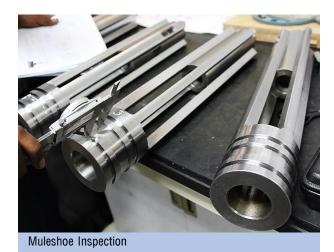
Instrument Barrel Assembly Muleshoe Sub Muleshoe Key Muleshoe Sleeve Stinger
