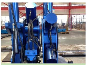
Screwing Tong Rotary Device
