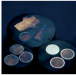
Crosscuts to check hardening depth.
