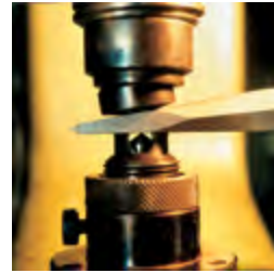
Special tool control for blade hardness.
