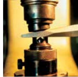
Special tool control for blade hardness.
