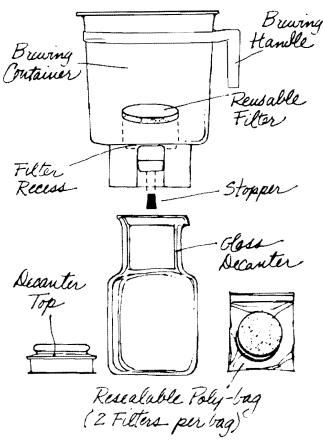
Brewing container - plastic (high density polyethylene) Brewing handle - plastic (high density polyethylene) Decanter - glass Filter - polyester
