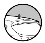
**SUV/Van/Hatchback:** Cable routed into top of hatchback door.
