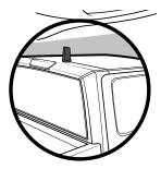
**Truck:** Cable routed into side door.
