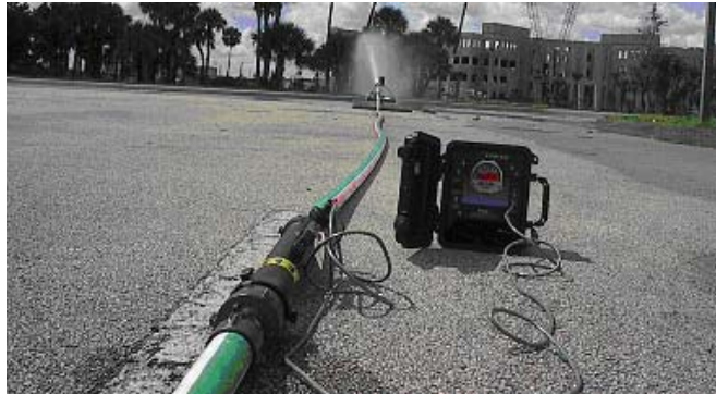
Friction loss testing of 1 3/4” Hi-Combat hose
