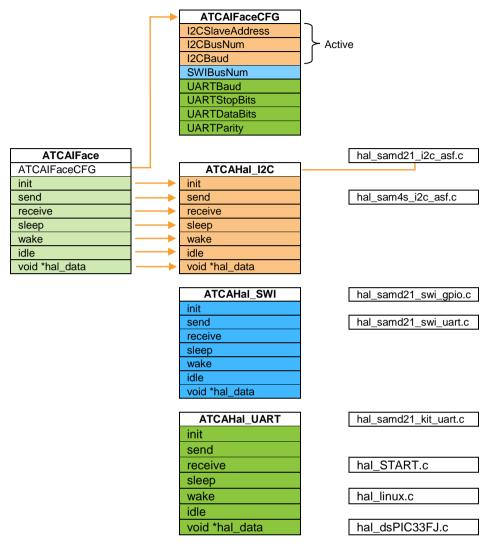
From the above diagram, there could be one of many different physical HAL implementations that are compatible with an ATCAIface object. That is the purpose of the HAL; to implement the methods in ATCAIface in a way that the client of the ATAIface object is unaware of the physical implementation used to communicate to the device.
