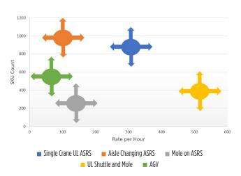
**FIGURE 3:** Unit load ASRS general selection based on SKU count and throughput. System throughput and SKU count are important considerations when selecting pallet-picking technology.
