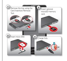
Insert the pin on the Card Insertion/Removal Tool into the hole in the tray to release the tray. Then, slide the tray out of the smartphone.
