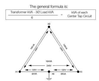
Note: All SolaHD 480 delta to 240 delta transformers stocked by Emerson are equipped with a center tap.
