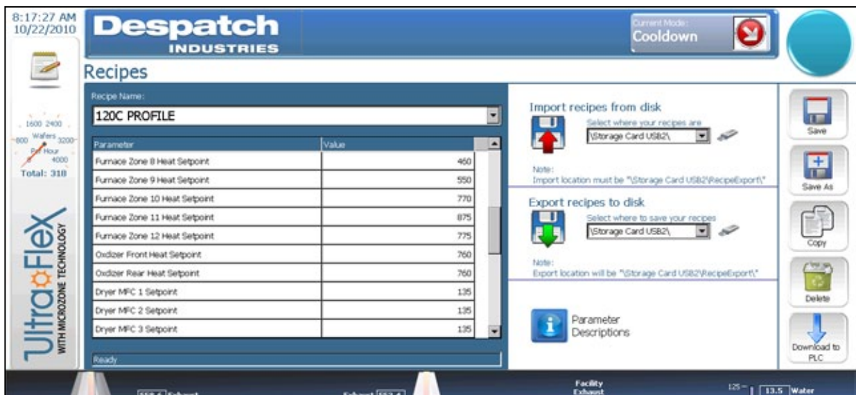
Figure 5. Set Four Dryer Process Air MFCs Using the Recipe Screen.
