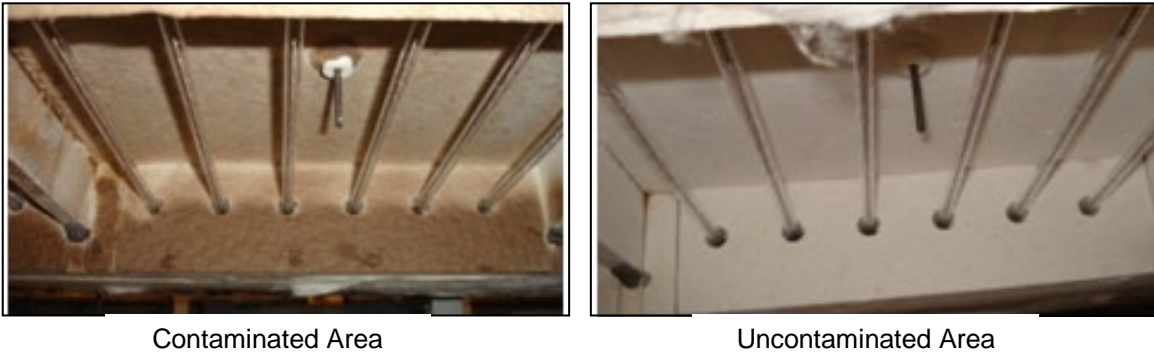
Figure 67. Contaminated Dryer Zone Before (left) and After (right) Insulation Burn-off procedure.
