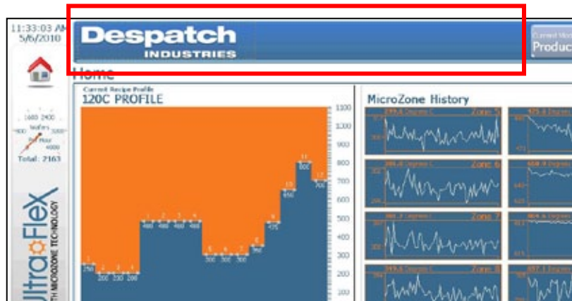
Figure 52. Press the Despatch Logo to Create a Screen Shot on the USB stick.
