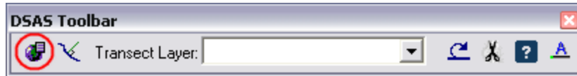
Figure 16. Screenshot showing the DSAS Toolbar application. The circled button launches the Set Default Parameters window.
