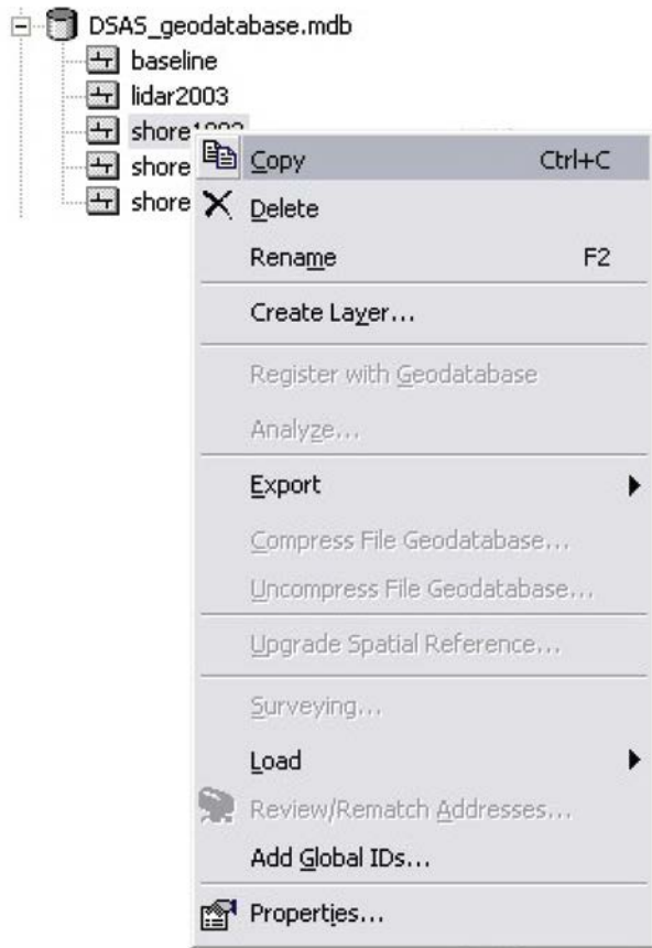
Figure 10. To make a copy of an existing shoreline, right-click on the feature class in the ArcCatalog file tree. Choose Copy from the popup window. Right-click on the geodatabase and choose Paste to specify where the copy should be placed. These actions will generate the window depicted in figure 11 .
