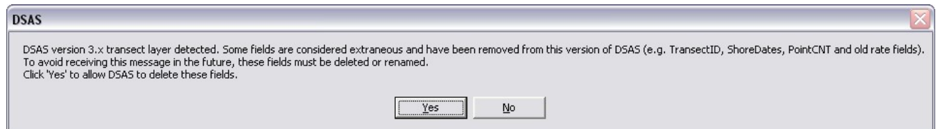
Figure 28. Screenshot of warning message that users may encounter when DSAS recognizes transects from previous versions of DSAS. This message will appear if any of the extraneous fields listed in the message are detected in the transect feature class attribute table.
