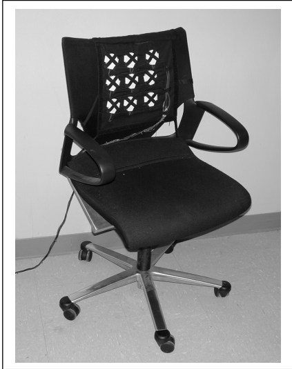
Figure 3. Experimental apparatus. Shown here is an office chair fitted with the 3-by-3 tactor array. Each tactor, enclosed in a white case, is fastened to a piece of fabric with two crisscross elastic bands.
