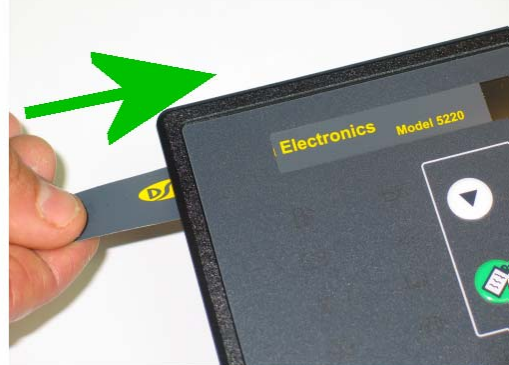
Removal and insertion of the Logo insert card
