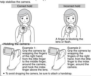
Make sure that the lens and flash unit are not blocked by your fingers or the handstrap. And do not block the built-in microphone on the monitor unit with vour hand.
