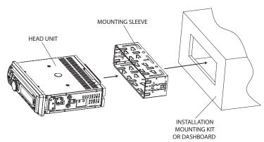
TYPICAL FRONT-LOAD DIN MOUNTING METHOD
