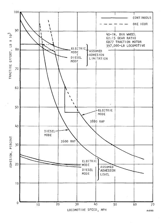
Figure 6. Tractive Effort-Speed Characteristics for SD40-2 Based DML
