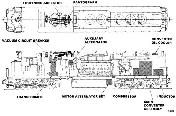
Figure 4. 25-kv DML, Equipment Layout
