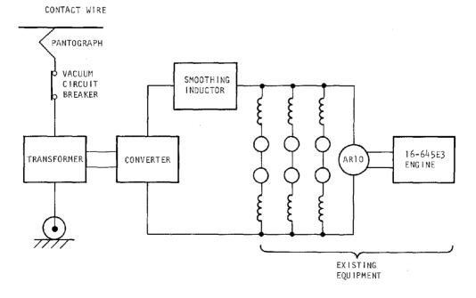
Figure 2. Simplified DML System Diagram
