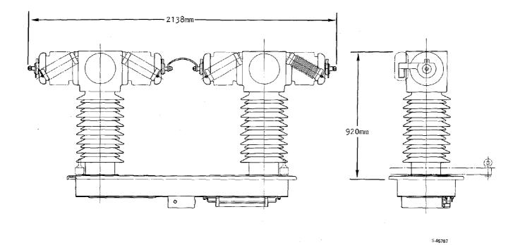
Figure 13. 50-kv Vacuum Circuit Breaker
