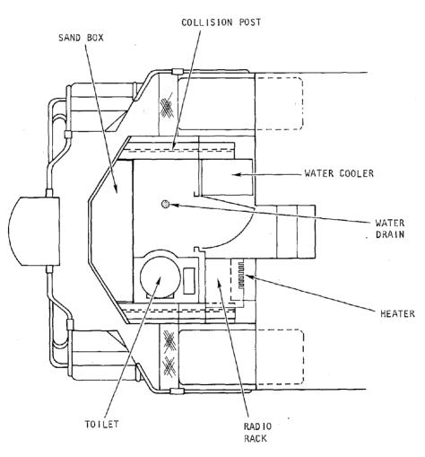
Figure A-1. DML Short Hood Arrangement
