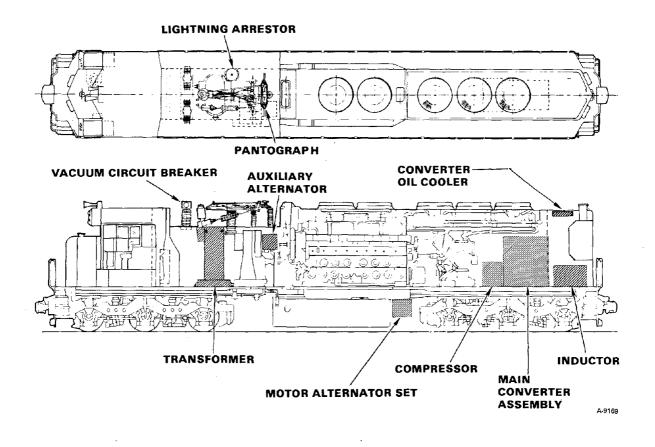
Figure 3. 50-kv DML, Equipment Layout
