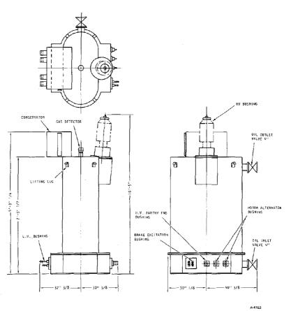
Figure 16. 50-kv Transformer
