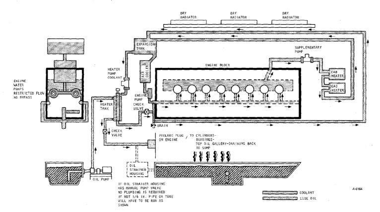
Figure 17. Typical Kim Hotstart Two-Fluid System
