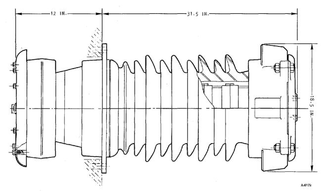
Figure 14. Typical Lightning Arrestor
