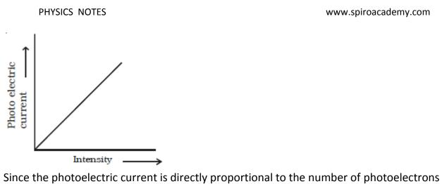
Since the photoelectric current is directly proportional to the number of photoelectrons emitted per second, it implies that the number of photoelectrons emitted per second is proportional to the intensity of incident radiation.
