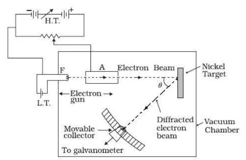
It consists of an electron gun which comprises of a tungsten filament F, coated with barium oxide and heated by a low voltage power supply (L.T. or battery).
