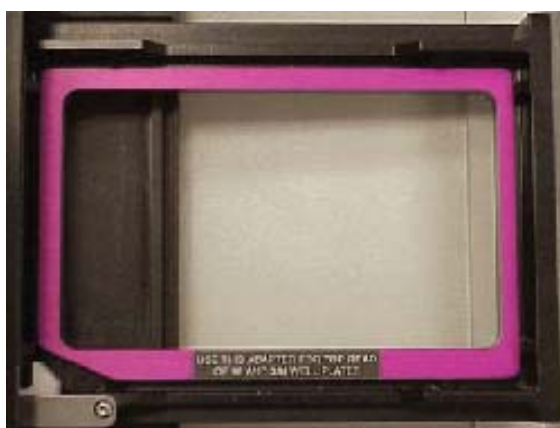
Figure 3.1: Adapter inserted in microplate drawer.
