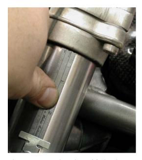
Fig 1. Measure location of fork tube.
