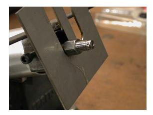
Fig 6. Top of rod with orifice.
