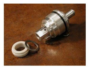
Fig 7. Upper plug assy. Note small parts.
