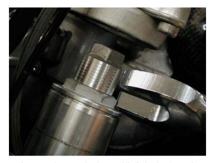
Fig 2. Break upper plug loose while fork tube clamped.
