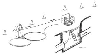
**WARNING:** Before pulling cable directly from a figure-eight, make sure that the area inside the loops of the cable is clear of personnel and equipment. Failure to do so may result in injury to personnel or damage to the cable.
