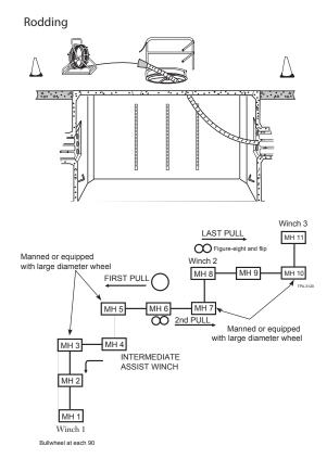
Inspect potential reel and winch locations for their suitability and make plans for installation techniques such as backfeeding or use of intermediate assist winches.
