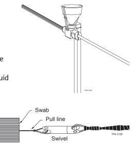
The use of a breakaway link (swivel) can be used to ensure that the maximum tension of the cable is not exceeded. Breakaway links react to tension at the pulling eye and should be used as a fail-safe rather than a primary means of monitoring tension.
