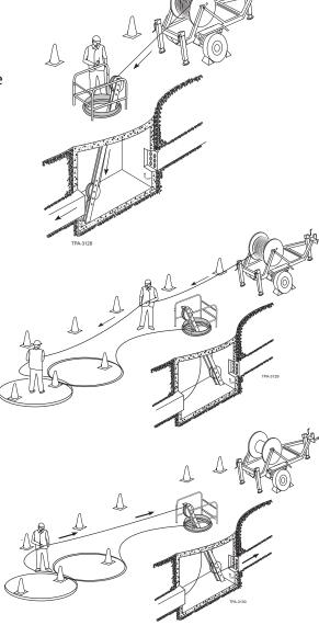
**Step 2:** After the pulling eye is connected to the next section of the pull-line, feed the cable by hand back into the manhole and pull it to its next destination. The cable may be pulled directly from a figure-eight by a winch, provided the capstan or sheave used at the entry manhole ensures sufficient bend radius. Hand tending of cable paying off from figure-eights is normally required.
