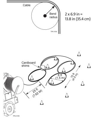
**WARNING:** Automated figure-eight machines that coil fiber optic cable on a drum may exceed cable design limits by exceeding torsion, tension, and bend radii limitations. Do not use automated figure-eight machines when installing fiber optic cables with a central tube design or any loose tube cable having one or more layers of corrugated steel armor. Use of these machines may result in the cable's jacket being breached and the armor being exposed.
