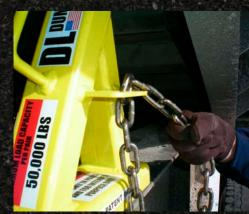
3. Slowly and carefully lower the dump bed to secure DUMP-LOK.
