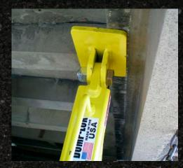
Place safety chain around truck frame or frame cross member. Slide chain through key slot hole. Tighten and lock chain in the small end of the slot. Repeat procedure for passenger side.
