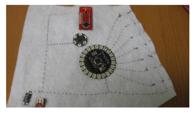
Make sure that your thread ends are cut nice and short next to the switch. It's important that the thread on one side of each switch not come in contact with the thread on the other side.
