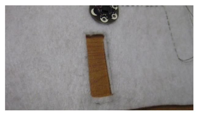
The side of the fabric you've laid the parts out on will be the back of the bracer. Press the display through the hole in the back to the front, like so.
