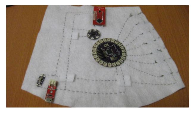
Here's that portion finished, with the felt bridges in place. Now, you've got your switches connected entirely, and you've got power and ground attached to all of your boards. You're missing an input from the accelerometer to the Arduino and an output from the Arduino to the serial display, so we'll do that next.
