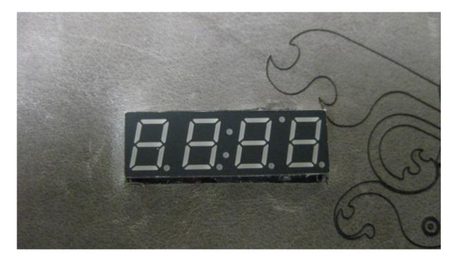
Once you've got your hole cut, **press the serial display through** it. You should have the display on the front of the leather, and all of the rest of the electronics on the back side, still exposed and visible if you flip the whole thing over. At this point, I put a few dabs of hot glue on the red board to secure it to the back of the leather and keep things in the same place so that, when I cut the next holes, they'll be lined up properly.
